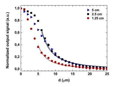
The response of the intensity with the displacement varies in accordance with the inverse square law accordingly with the equation:
