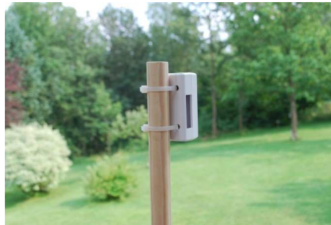
Figure 2.1: A mote mounted on a wooden pole
