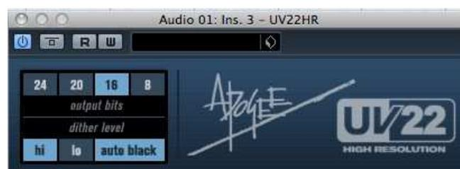
Figura 71: Apogee's UV22 High Resolution dithering plug-in.
