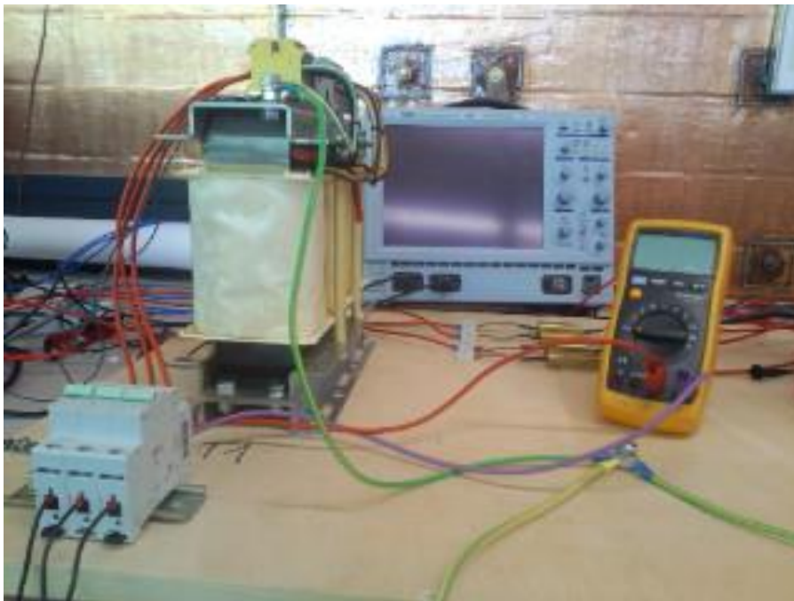
Figure 15: Short-circuit test setup
