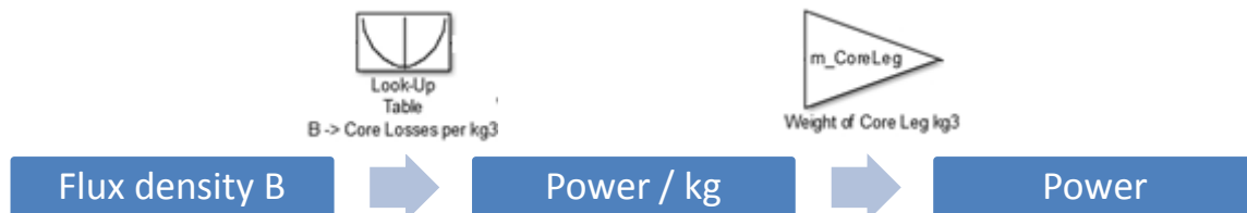
Figure 6: Simplified iron losses computation by the model for a core segment
