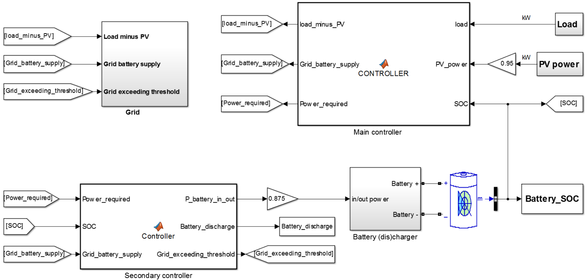
Figure 55: Simulink model of the whole system
