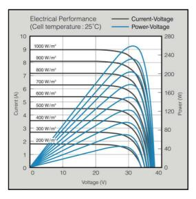
Figure 4.I-V, P-V, for different values of irradiance. Source: Mitsubishi Electric.
