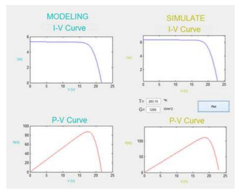
Figure 7. Results of the KC85T solar panel (35°C and 1200W/m<sup>2</sup>) with method 1.
