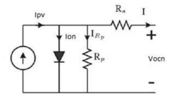
Figure 5. Single-diode model accounting for ohmic losses.
