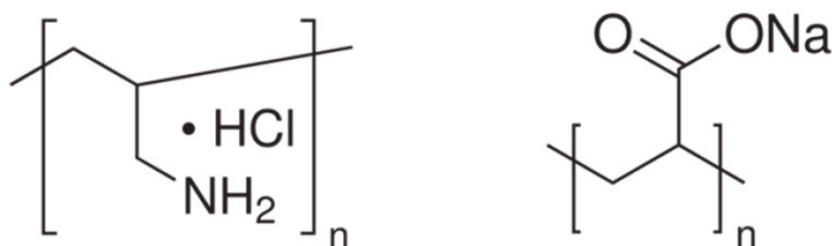
Figure Ap2.2. Chemical structure of both cationic and anionic polyelectrolytes (PAH and PAA).
