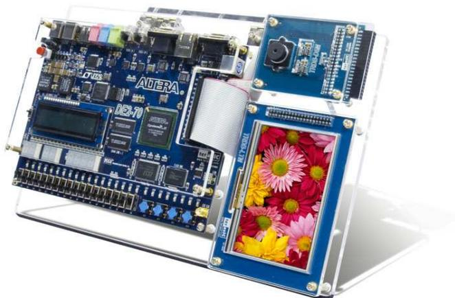
**Figura 1. Kit DE2-70 + Cámara Digital 5M + Panel LCD**
