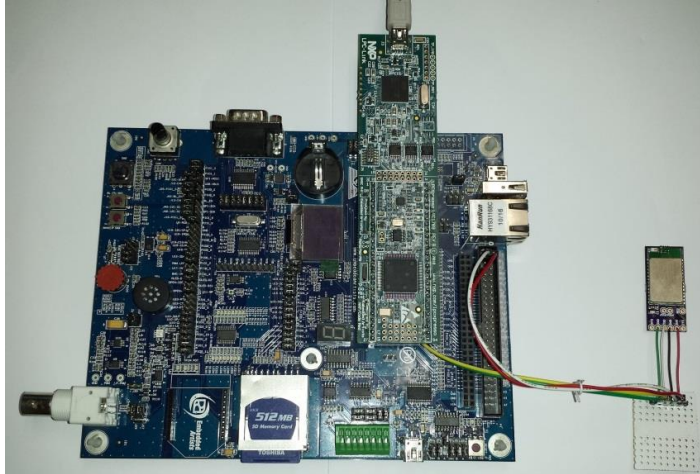
Figure 5.2: Agent: LPC1769 development board and Breaking Board.
