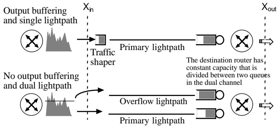
Figure 5: WDM link model with overflow channels
