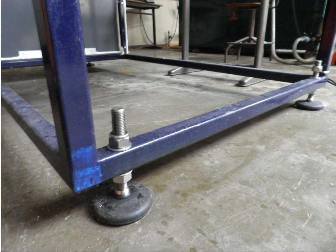
Pic. 59 The legs are adjustable, so we can increase the height (10 mm.) easily.
