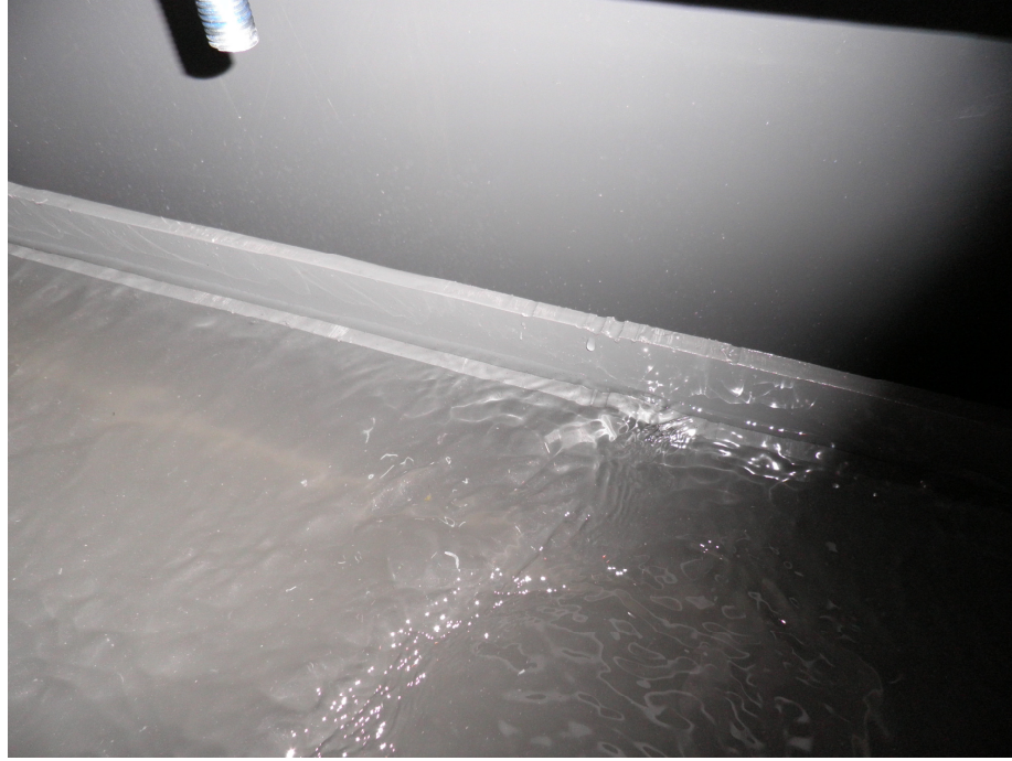
Pic. 7 Some amount of flow goes back by the gaps in the sides of the opening
