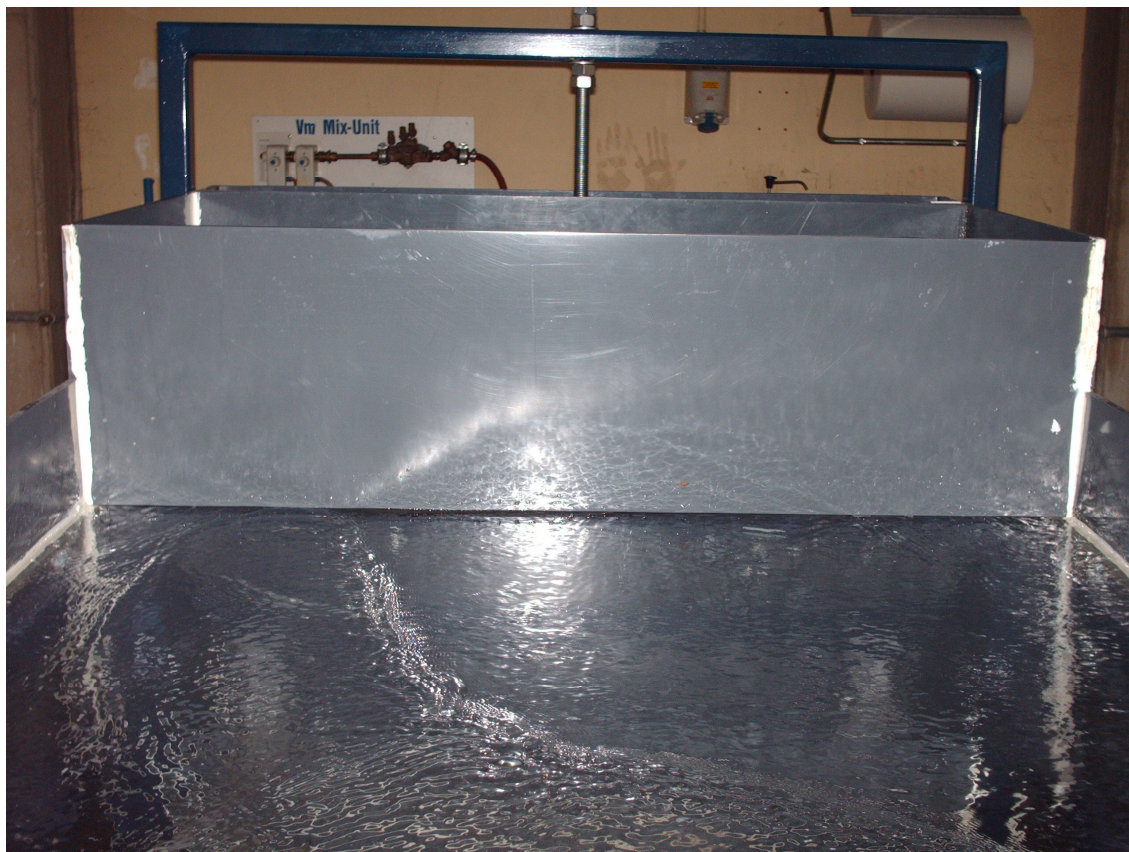
Pic. 10 Two pumps working: Turbulences without the grille installed.
