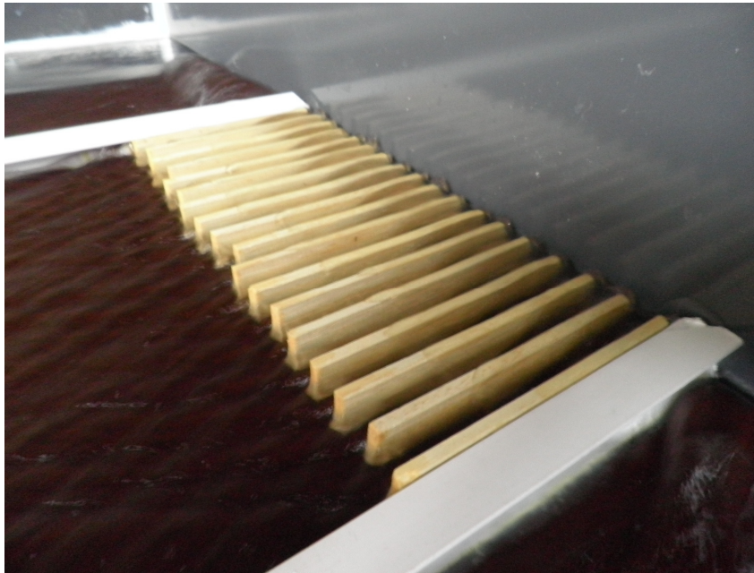
Pic. 46 After the tracks thin oblique lines appear in the water, but they are very soft and they do not affect the flow.
