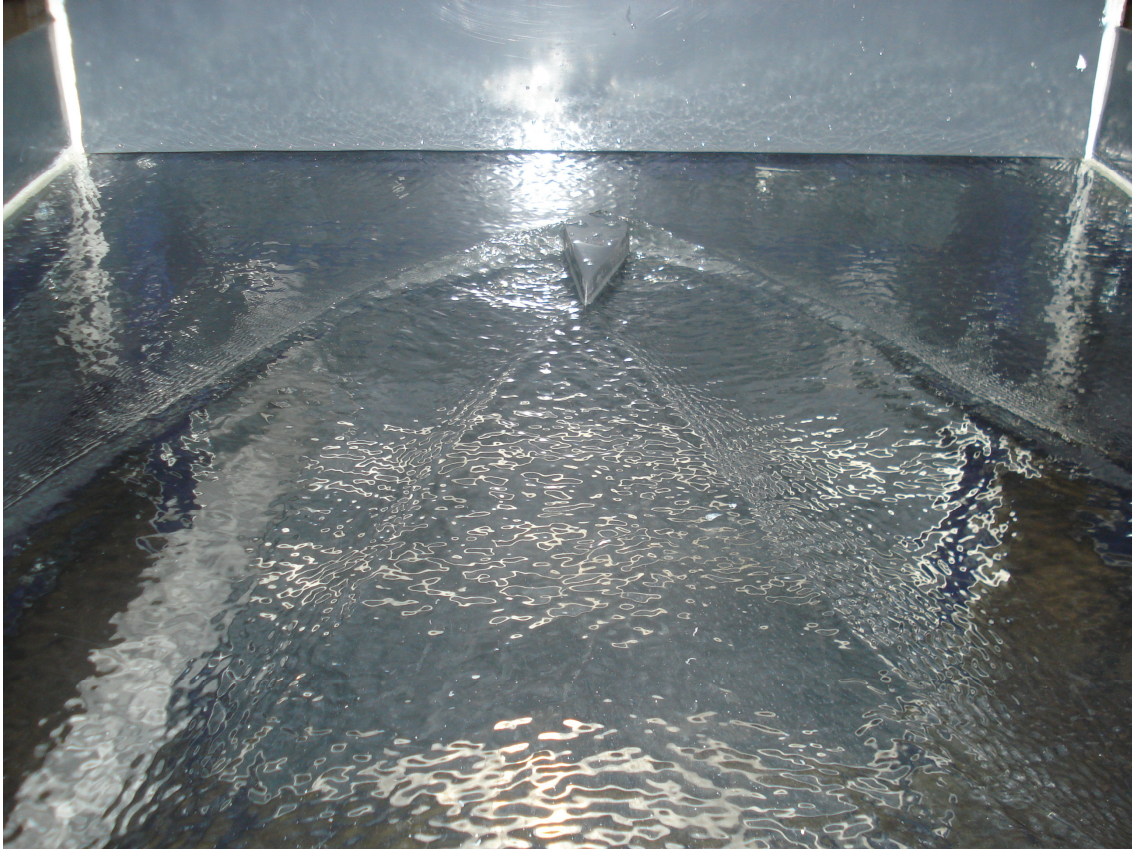
Pic. 11 Two pumps working (with the grille installed): The turbulences have decreased and we can visualize shock waves in blunt bodies in a better way than before (it is not already a good result but it is better than without the grille).
