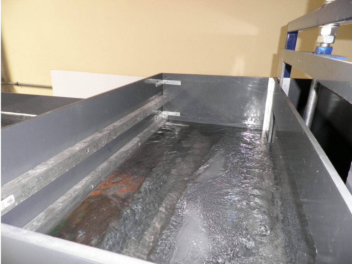
Pic. 24 At the right part of the picture it can be seen the opening completely closed and at the left part the height (60 mm.) of the mass of water.
