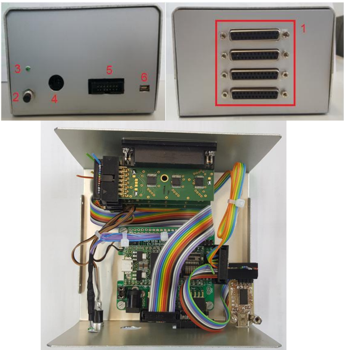
Figure 4.10 - Metallic box with master FPGA and shift register
