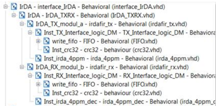
Figure 8.5 - IrDA interface VHDL code hierarchy
