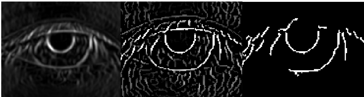
Figure 5.8: From left to right, Edge map obtained using canny method, non-maxima suppression image, hysteresis thresholded image.
