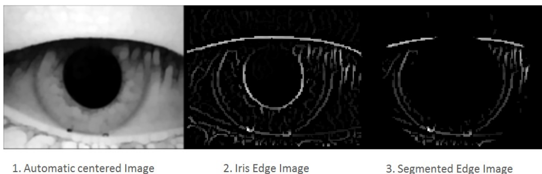
Figure 5.15: Selection of the Edge Map using the information of the iris radius and the position of the pupil centre
