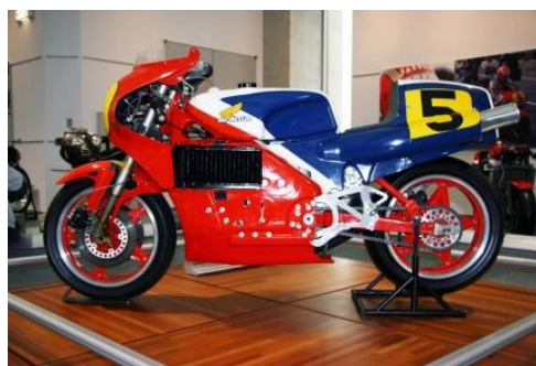
Figura 4.23-Honda NR500, chasis monocasco
