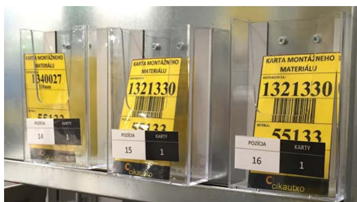
Picture 46 - Real holders with it kanban cards
