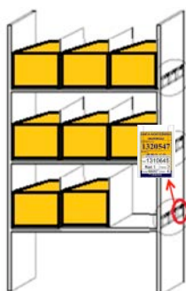
Picture 55 - Kanban card in the holder of the rack
