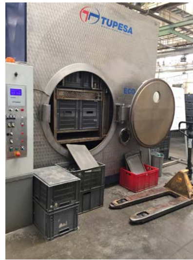
Picture 27 - Boxes inside the washing machine
