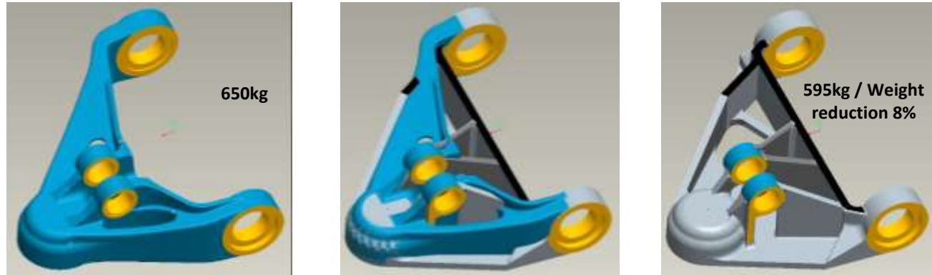
FIGURE 31.- Comparison between former design of the control arm and CAD geometry of the concept design in Pro/ENGINEER
