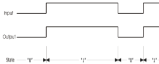
Figure 4.10 - Signal Diagram of Digital Inputs/Outputs
