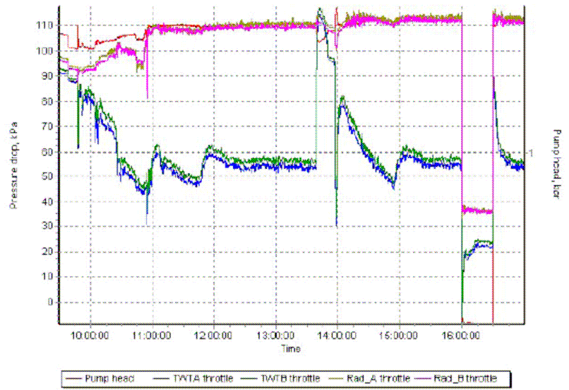
Change of pump head and pressure drop on MPL components
