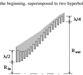
$\alpha$  being a value approximately of 1.3 which controls de taper slope, L the total length which is calculated to achieve the correct output radius (between  $0.7\lambda$  and  $0.8\lambda$ ) to obtain approximately the mixture of 85% of TE<sub>11</sub> and 15% of TM<sub>11</sub>, the phase will be automatically adjusted. This means, there are a lot of possibilities, and we have to choose the best one for our particular application.
