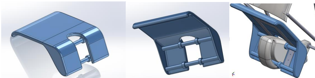
Fig.5.24: complete seat views and riveted plate
