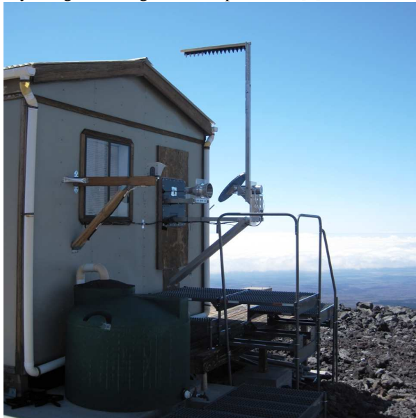
Fig.1: Water Vapor Millimeter-wave Spectrometer (WVMS-5) under operation at Mauna Loa Observatory (Hawaii)
