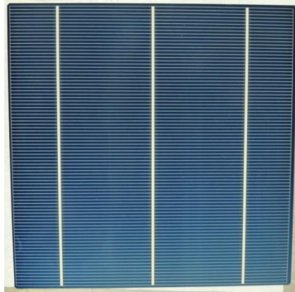
Figure 33. Results of front side metallization of standard Al-BSF solar cells with and without rear soldering pads
