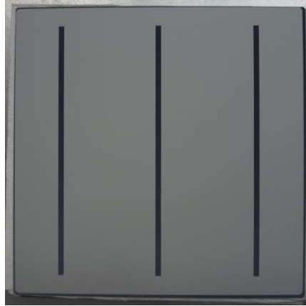
Figure 37 . Result of screen printing of the aluminium layer on standard Al-BSF solar cells with soldering pads
