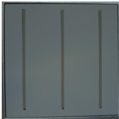
Figure 39. Picture of the rear side of one of the metallized wafers after having the rear busbars printed
