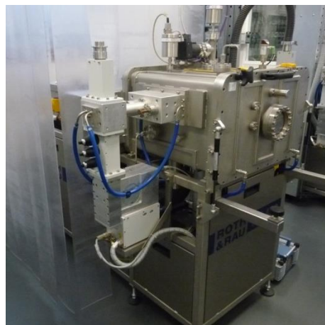
Figure 18 . PECVD equipment for silicon nitride deposition [CENER]
