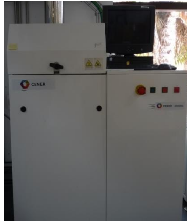
Figure 22. RTP equipment [CENER]
