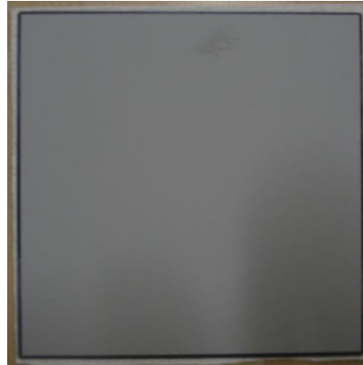
Figure 35 . Result of rear side metallization of standard Al-BSF solar cells without soldering pads
