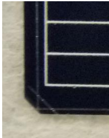
Figure 42. Detail of the laser edge isolation process performed for the solar cells
