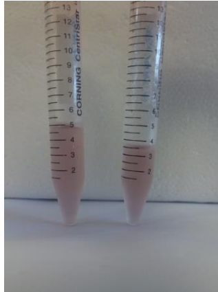
Figure F : Au-Gel2 nanoparticles batch at 6 \cdot 10^{-6} \mu\text{mol NP4/mg gelatin} after purification at 2k (discarded) and 14k (suitable) from left to right.
