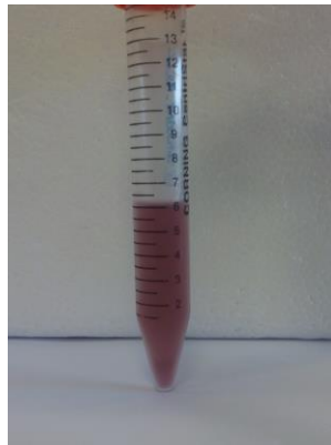
Figure G : Au-Gel2 nanoparticles batch at 12 \cdot 10^{-6} \mu\text{mol NP4/mg gelatin} after purification at 14 k (suitable).
