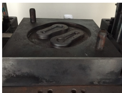
Figure 4. Set of dies used in the manufacturing of the connecting rods.
