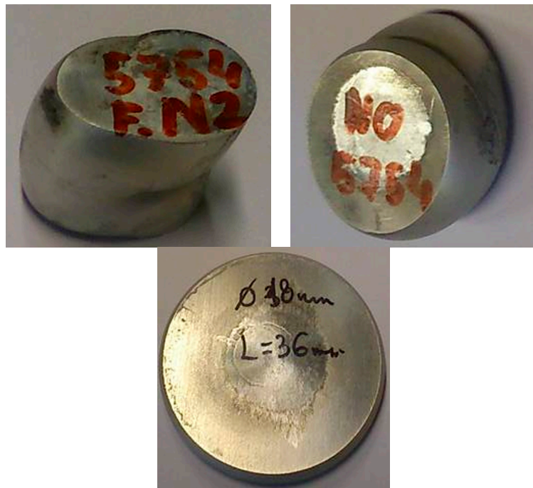
Figure 13. Billets with buckling and final test without buckling.
