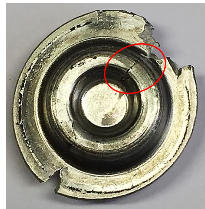
(b). Preform and connecting rod forged at 200 °C from N2 AA5754
