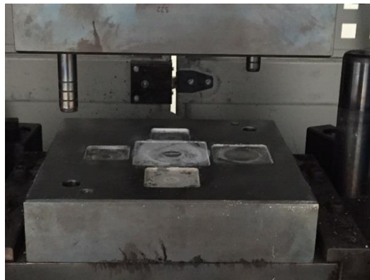
Figure 9. Set of dies employed to perform the isothermal compressions
