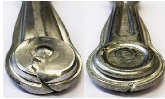
(b). Preform and connecting rod forged at 200 °C from N2 AA5754
