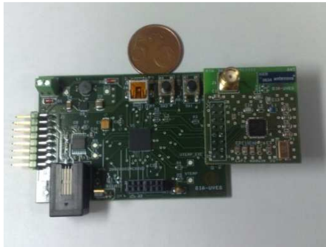
Figure 4.3. Image of the main board (left) and the radio frequency module (right) of the mote device.
