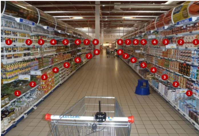
Figure 3.75. Real scenario. Note that the shelves on the left are filled mainly with products in glass jars, and the shelves on the right with products in metallic cans. Numbered red dots represent the measurement points.
