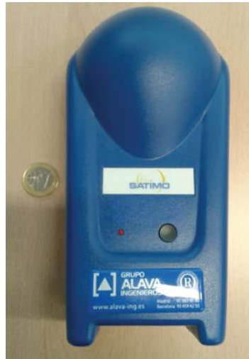
Figure 5.29. The EME Spy 121 dosimeter used to obtain electric field values of the leakage of the microwave oven.
