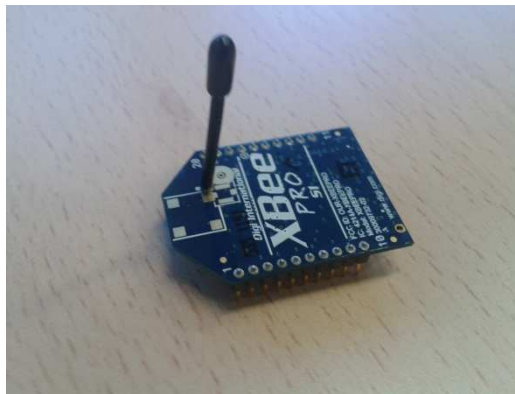
Figure 3.38. The ZigBee mote used for ZigBee wireless communications inside the car.
