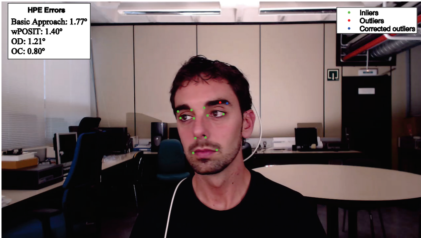
Figure 4.11: Visual example of the effect of the OC module on a frame from the UPNA database. Inliers are represented in green, the outlier detected by the OD module in red, and the corrected point estimated by the OC module in blue. Instantaneous HPE errors of the four approaches are shown on the top left side.
