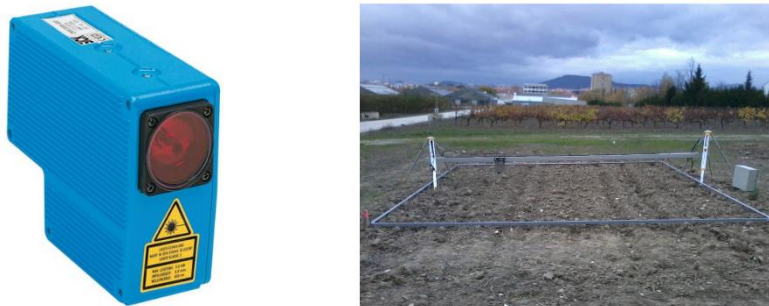
Fig. 2.2. SICK DME 2000 laser sensor (left) of the profilometer (right) used for data taking.
