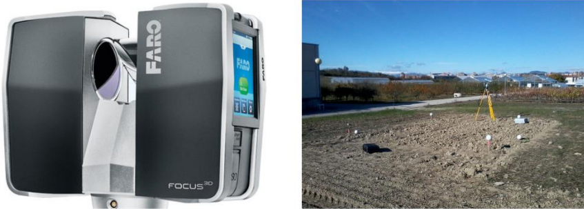
Fig. 2.4. FARO focus 3D (left) and the scanning setup (right) used for data acquisition.
