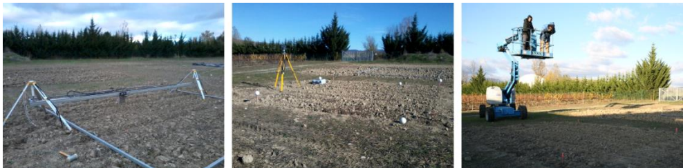
Fig. 6.2. Measurement techniques: Laser profilometer (left), Structure for Motion (center) and Terrestrial Laser Scanner (right).
