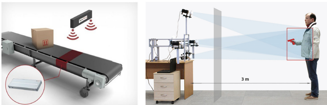
Figure 3.16. Layout for linear THz imaging system installation on a conveyor (left) and THz security body scanner (right).
