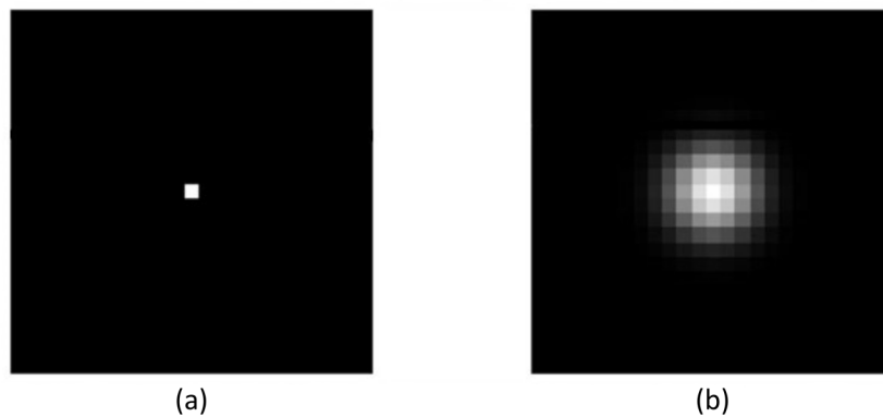
Figure 2.9. (a) Delta-like pixel and (b) the effect produced by the discrete convolution with the PSF.
