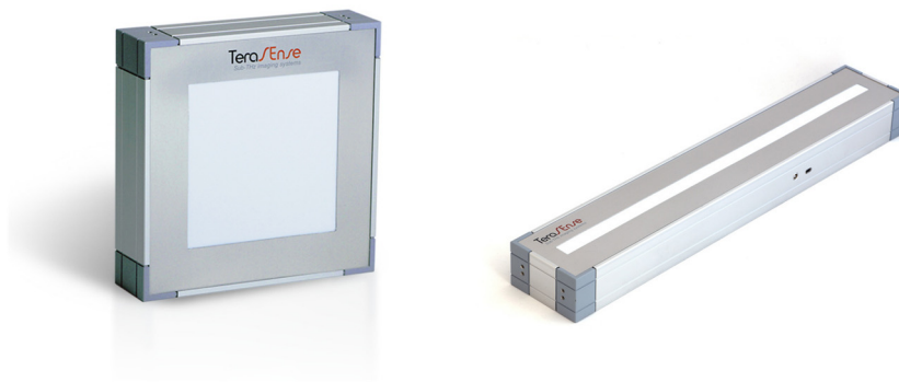
Figure 3.15. Terahertz imaging camera of 4096 pixels (64×64 array) and linear camera of 1024 pixels (256×4 array).
