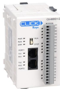
Figura 31 CPU PLC (Fuente [6])
