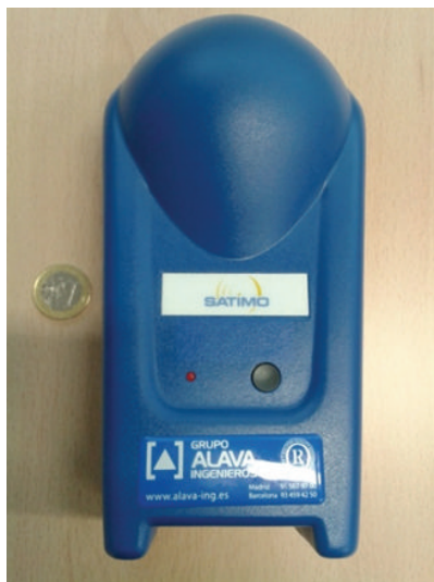
FIGURE 8: The EME Spy 121 dosimeter used to obtain electric field values of the leakage of the microwave oven.
