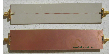
FIGURE 1: Photograph of the fabricated prototype in microstrip technology; top view of the metallic strip and bottom view of the unaltered ground plane.
