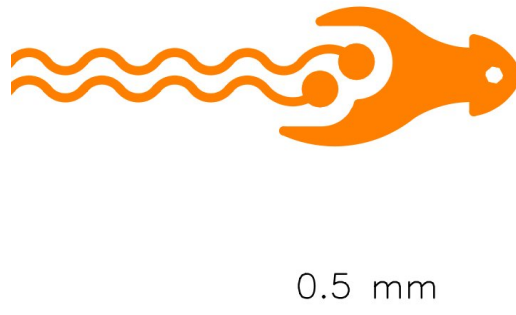
Figure 3.3: Second version of the electrode tip - Made wider and with a handling hole.
