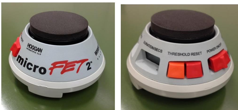
**Figura 30.** Dinamómetro digital Hoggan MicroFET 2 (*Hoggan Scientific L.L.C. Salt Lake City, Utah*).
