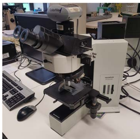
Fig. 20. Optical microscope employed for the fiber diameter measurements.
