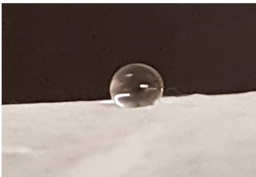
Fig. 28. Picture of a water drop deposited on a surface coated with electrospun PVC fibers. The high water repellency and WCA can be observed at a glance.
