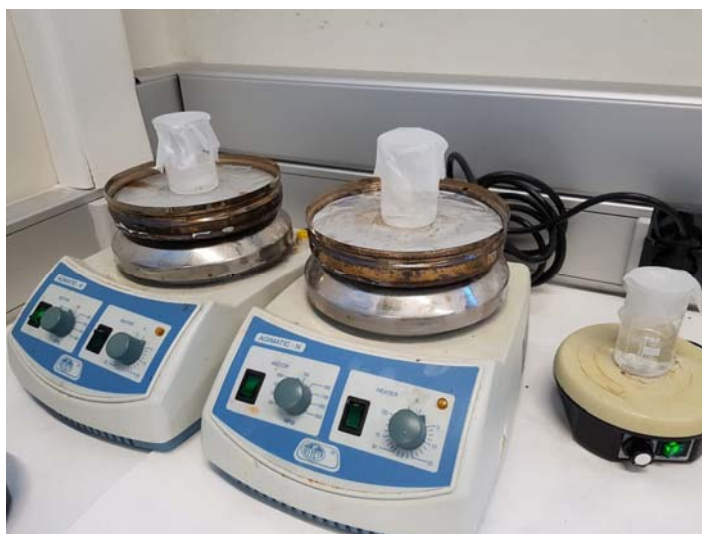
Fig. 15. Magnetic stirrer employed for the solution preparation.
