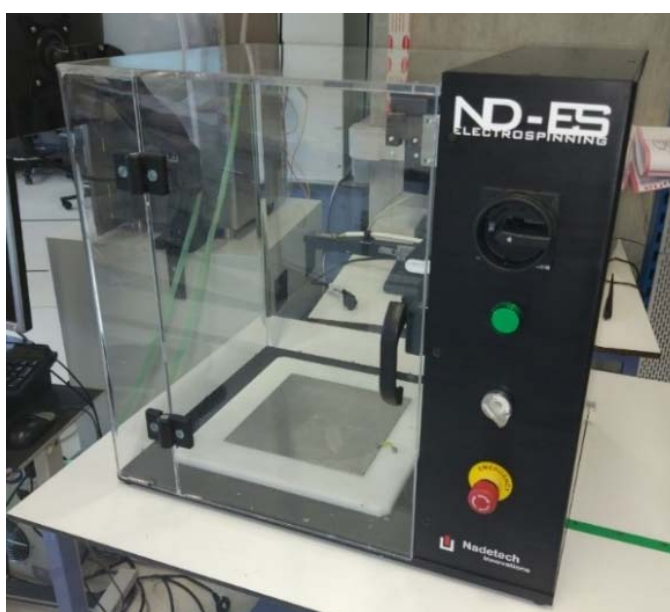
Fig. 17. Nadetech electrospinning equipment
