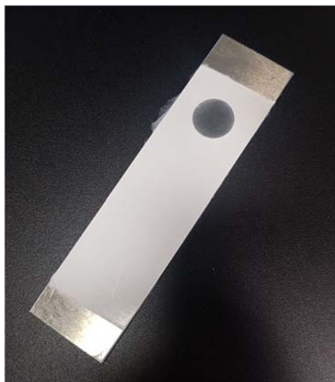
Fig. 54. Aluminum slide coated with electrospun PVC fibers before being heat-treated.
