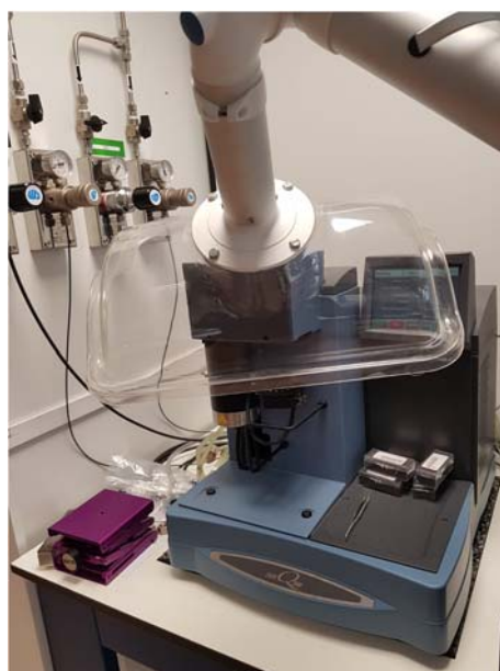
Fig. 30. Thermogravimetric analyzer of the AIN (Asociación de la Industria Navarra), where the TGA tests were performed.
