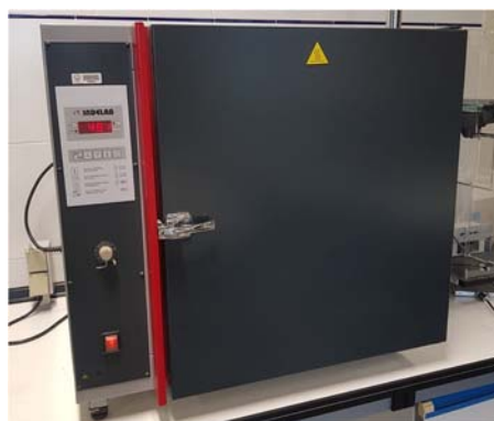
Fig. 40. Oven employed for the heat treatment of the samples.
