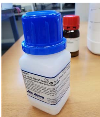
Fig.14. ZnO nanoparticles in colloidal dispersion, 50% in H_2O . Average particle size of 50 nm.
