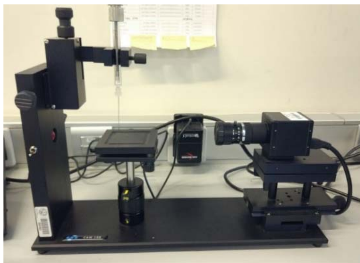
Fig. 25. CAM 100 contact angle goniometer employed for the WCA measurements.
