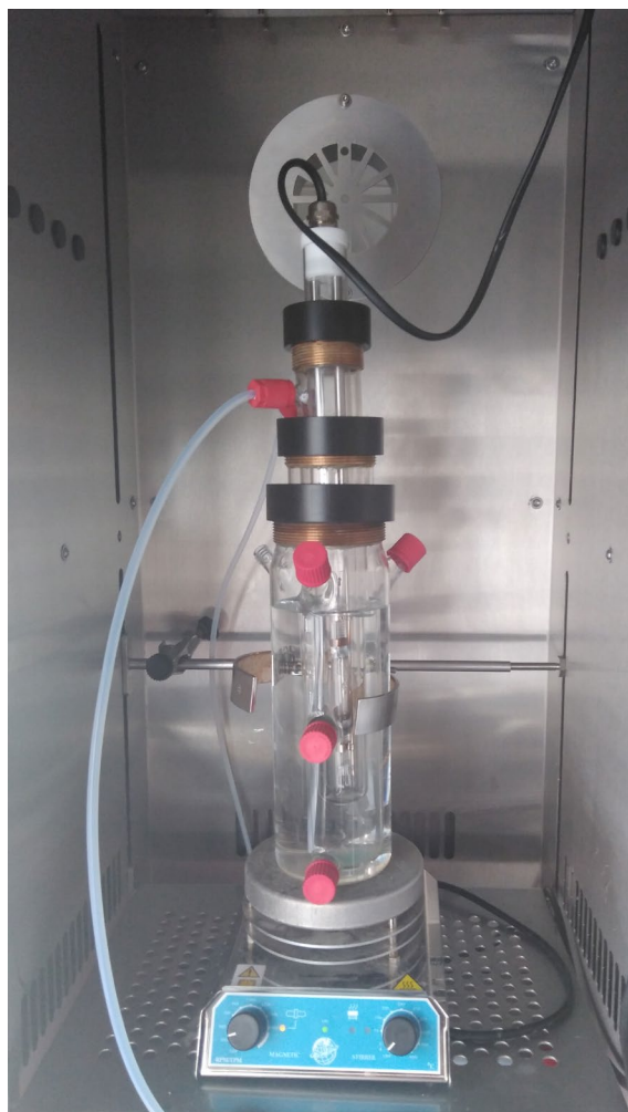
Fig. S1. Photograph of the photocatalytic reactor.
