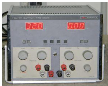
Figura 10. Fuente DC Power Supply FAC-662B
