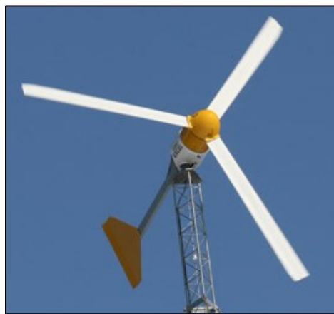
Figure 1.11 Small-scale (10 kW) wind turbine example [12]
