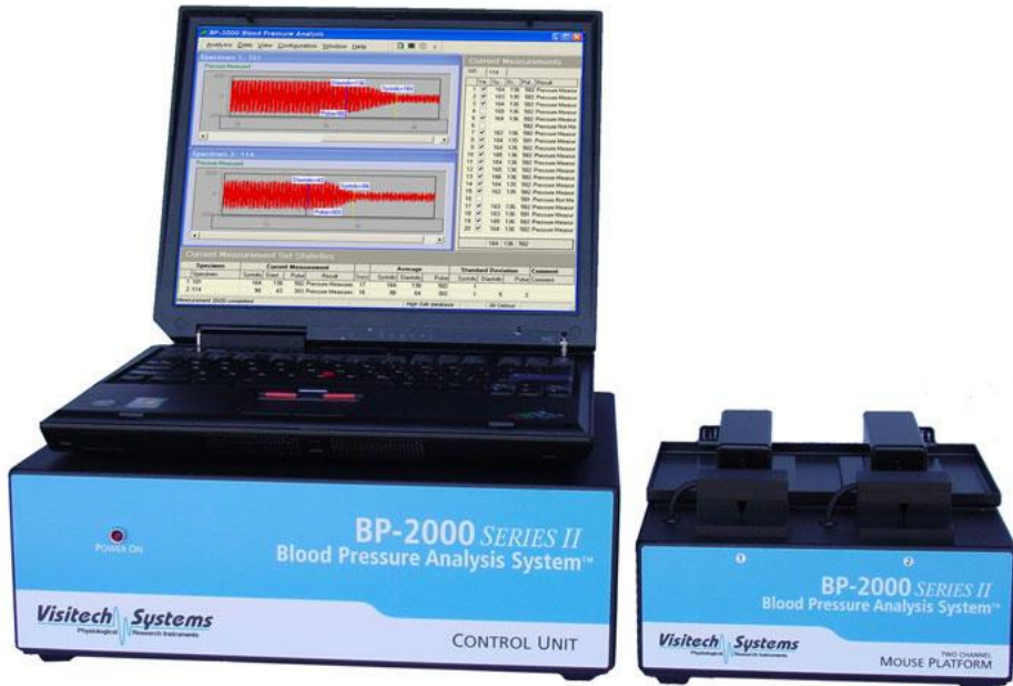
Figure 19. System for measuring blood pressure and heart rate. (BP-2000 SERIES II Blood Pressure Analysis System™, VISITECH, USA).
