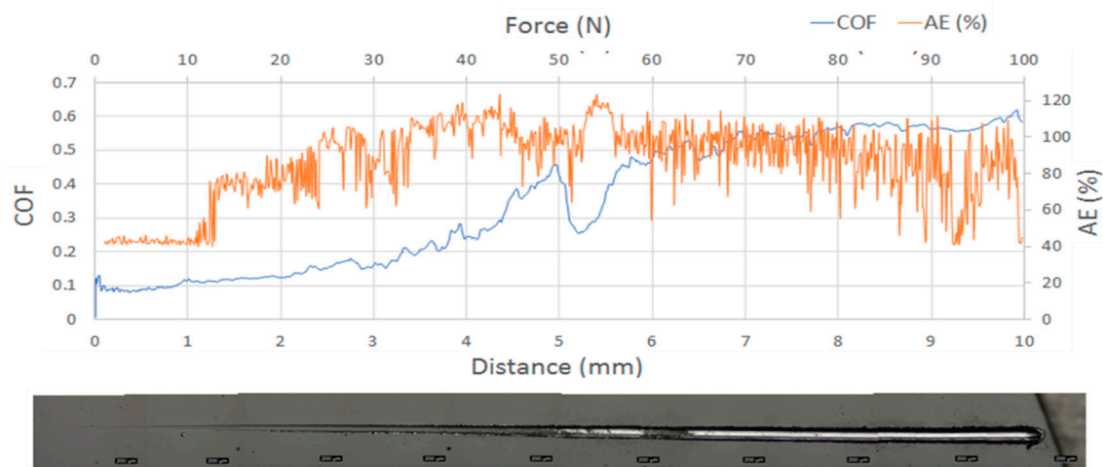
Figure 7. Nanoscratch test for ta-C coating. Evolution of the coefficient of friction (COF, blue plot) and the acoustic emission (AE, orange plot) vs. the indenter displacement, and optical micrograph of the scratch tracks.
