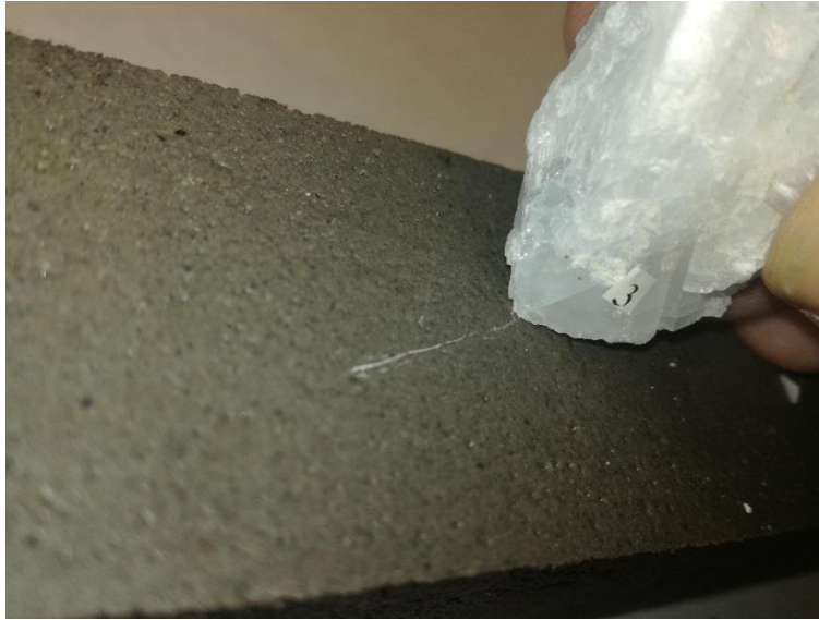
Figure 6. Procedure carried out for surface scratching test.
