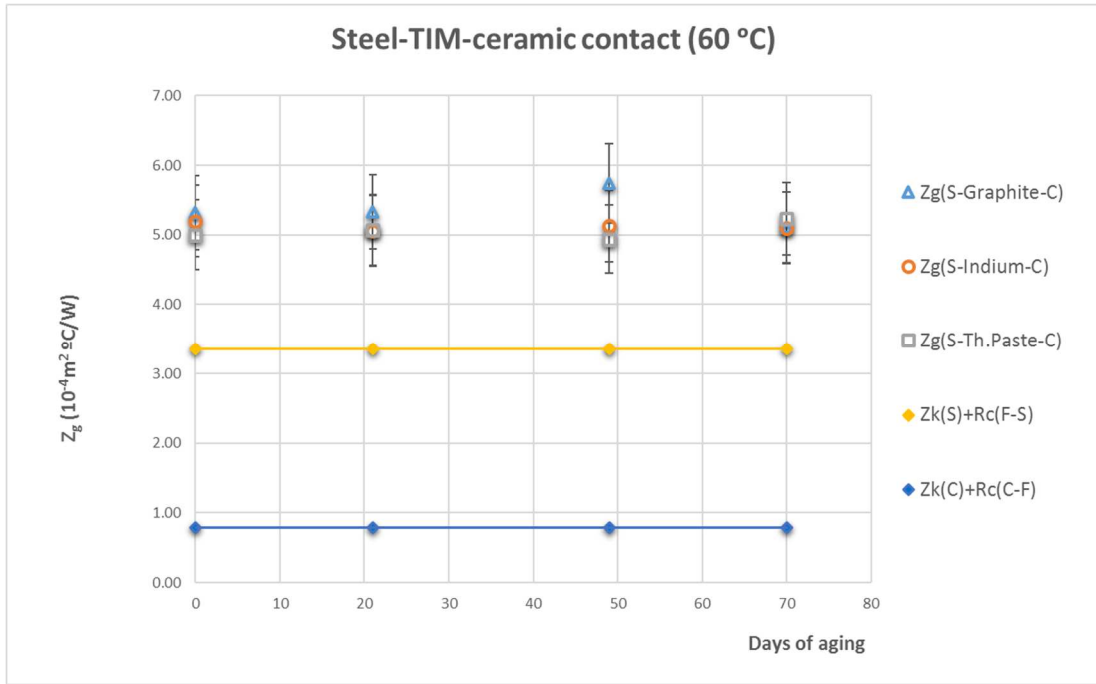
Fig. 10. Steel-TIM-ceramic contact ( 60^\circ\text{C} )
