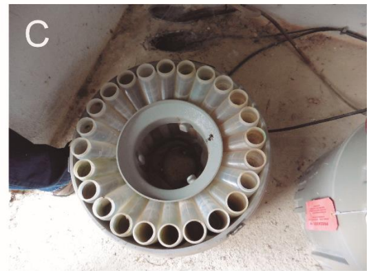
1011 Figure 3. (A) Hydrological station at the watershed outlet and hemispheric hollow, and (B, C) the 1012 automatic sampler.
