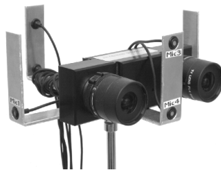
Figure 5.1.: Robot head with the microphones
