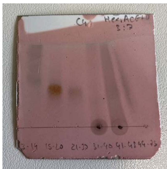
Figure 3. TLC of the fraction obtained by column chromatography applied to the DCM extract, revealed with anisaldehyde.
