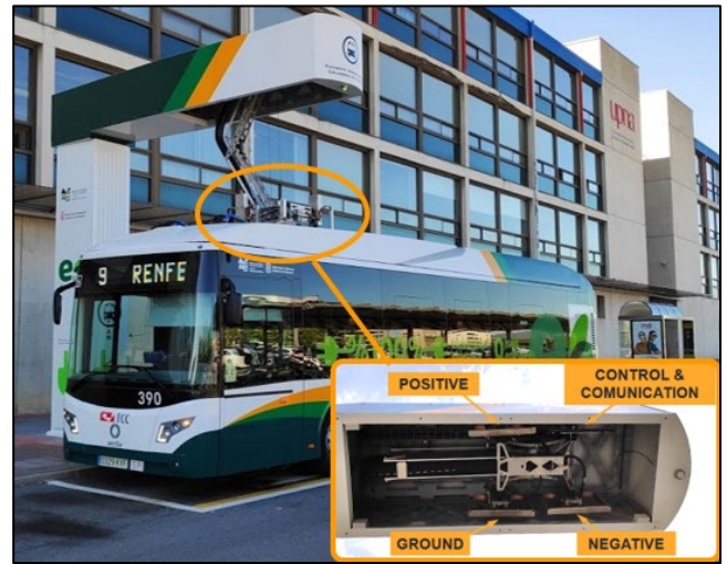
Fig. 1. Electric bus charging station located at Public University of Navarre. impact of the power peaks demanded from the grid during frequent recharging periods.
