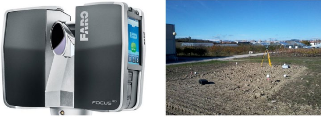
Fig. 1. FARO Focus 3D (left) and the scanning setup (right).
