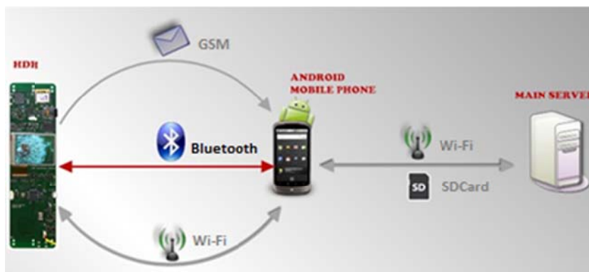
Figure 3.2 Bluetooth connection HDH-Android Server
