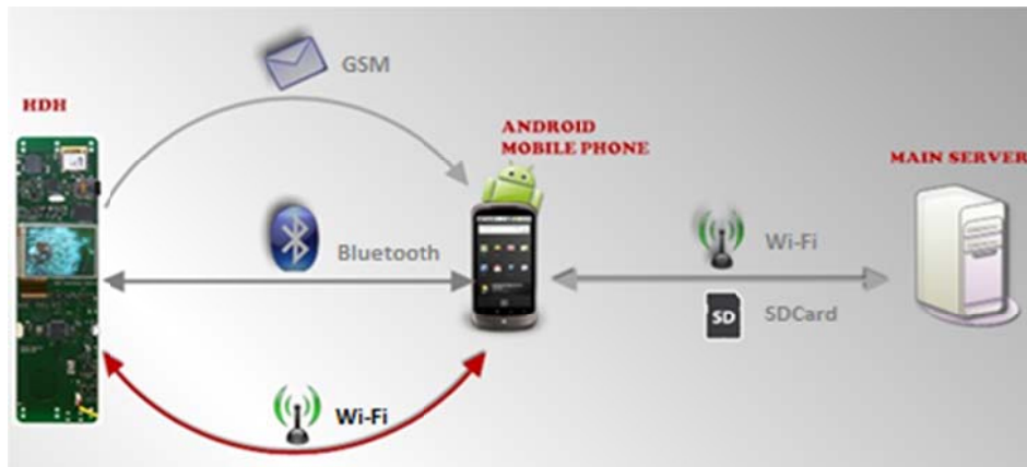
Figure 3.17 Wi-Fi connection HDH-Android Server
