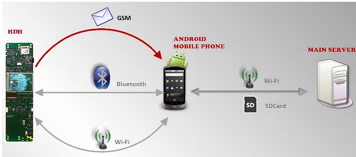
Figure 3.21 GSM connection HDH-Android Server
