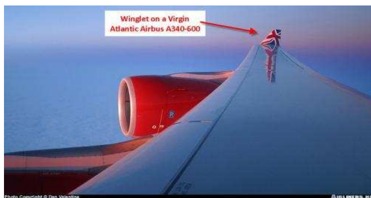
Fig.6: Winglets on a Virgin Atlantic Airbus A340-600.
